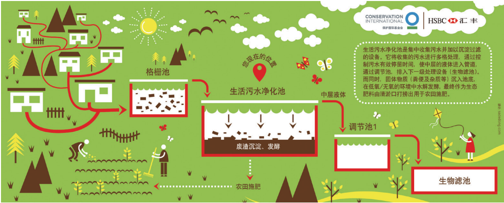
山区无动力污水处理系统示意图 Illustration of the Southwestern China Mountain Waste Water and Sewage Treatment System to Prevent Pollution to the Yangtze
